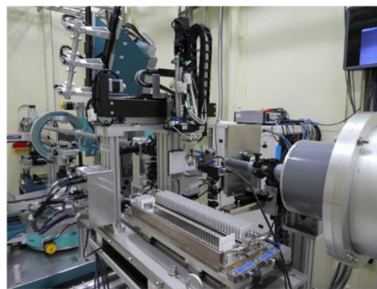
Fig. 3. Sample changer robot at BL08B2. Sample is shown in the beam position.
