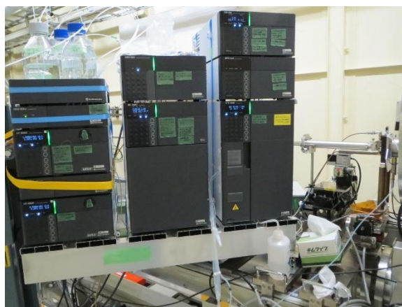
Fig. 1. Liquid chromatography system and SAXS measurement system at BL40B2.
