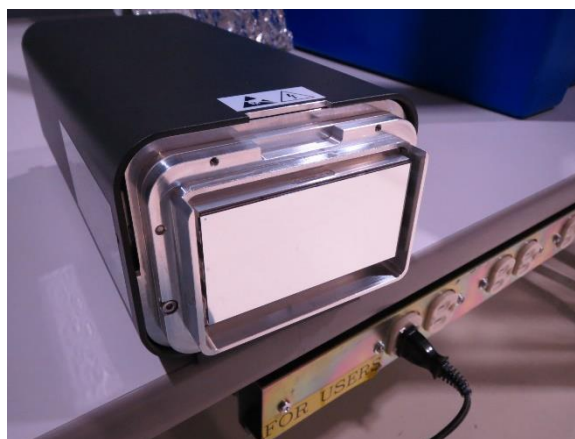
Fig. 2. WAXS detector with newly designed frame and housing.
