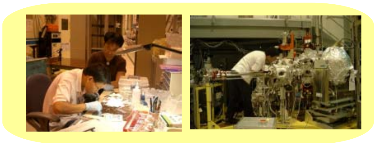
Fig. 2.2: (Left) Setting a sample on a sample carrier. (Right) Transferring the sample to the experimental station.
