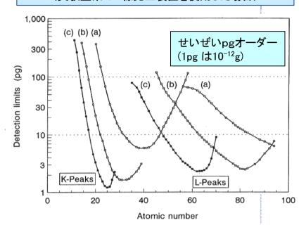
Detection limits of TXRF for the residues of aqueous solutions, dependent of the atomic number of the analyte element. Three excitation modes were used: (a) Wtube, 50kV; Ni-filter, cutoff 35keV; (b) Mo-tube, 50kV; Mo-filter, cutoff 20keV; (c) W-tube, 25kV; Cu-filter. The three curves to the left were determined by the detection of K-peaks; the three curves to the right, by that of L-peaks.
