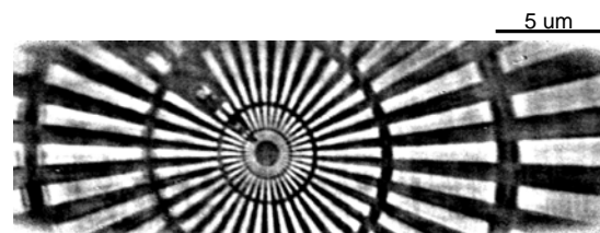
Fig. 2 Obtained bright field image of a Siemens star chart at an X-ray energy of 9.881 keV. A 100-nm feature is clearly visible.
