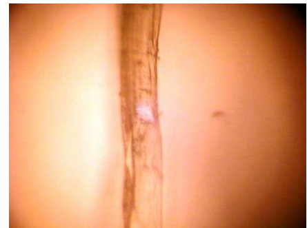
Fig. 2 Measured part of reference modern ramie fiber. Central highlighted point is an analyzed part.
