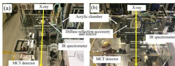
Fig. 1. XAFS-IR simultaneous measurement system: (a) before and (b) after improvement of acrylic chamber.
