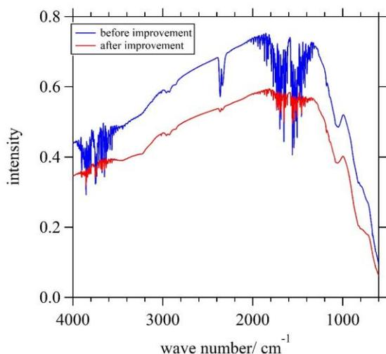
Fig. 2. IR spectra of the background measurement.
