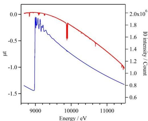
Fig. 3. Cu K-edge QXAFS spectrum of the Cu foil (blue line) and I0 spectrum (red line) measured using NF CA5350.
