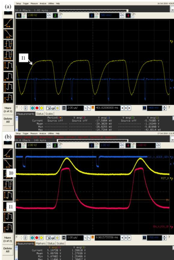
Fig. 5. Waveforms of (a) I1 (Yellow) Amp. Out signal of NF CA5350 and (b) I0 (Yellow) and I1 (Red) Amp. Out signals of FEMTO DLPCA-200. The blue lines of (a) and (b) are the trigger signals synchronized with each revolution of the electron bunch.
