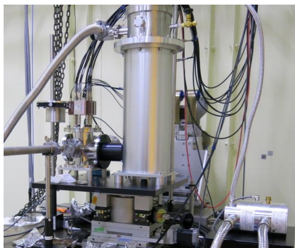
Fig. 2. Analyzer for energy domain Mössbauer spectroscopy with a closed-cycle cryostat.
