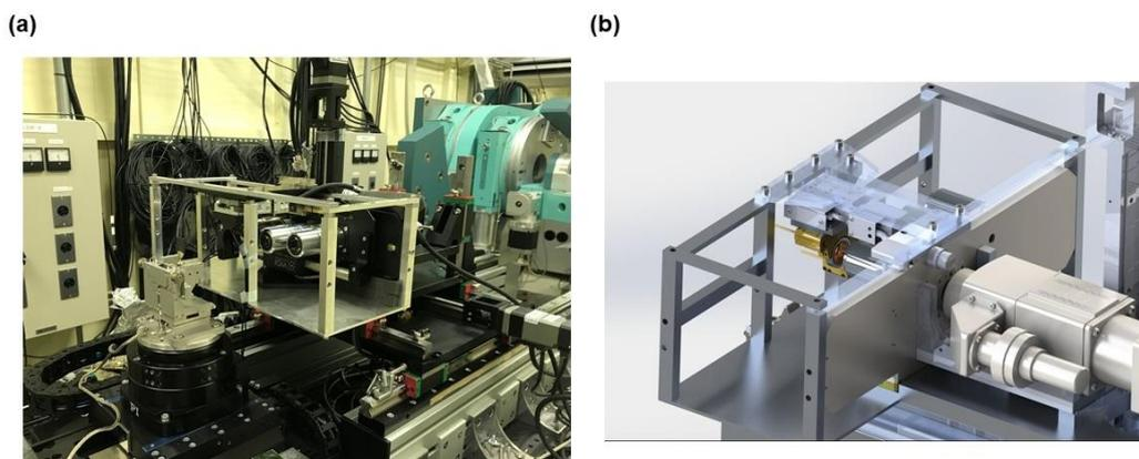
Fig. 2. Projection X-ray Microscopy (PXM) end station installed at BL12B2. (a) Photo and (b) schematic layout.
