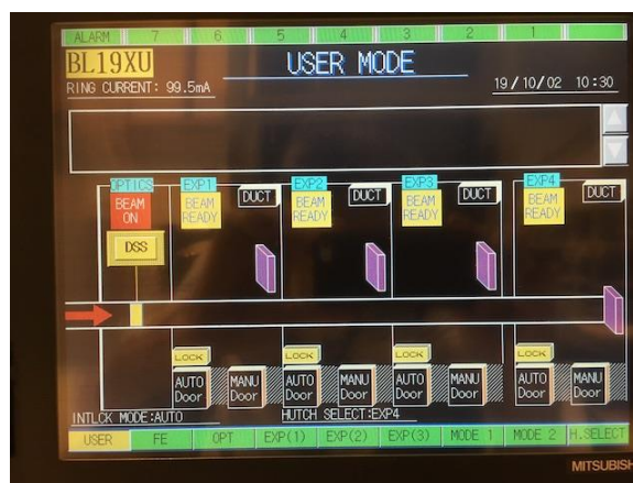
Fig. 1. Graphic panel of the new interlock system in the USER mode. MBS button is hidden to prevent users from closing MBS carelessly, and appears only when users can open it.
