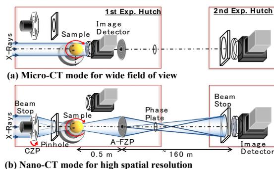
Fig. 1. Schematic drawing and typical parameters of multiscale CT at BL20XU.
