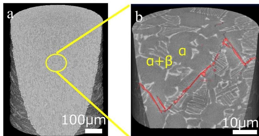
Fig. 2. Multiscale-CT images of interior fatigue cracks in Ti-4Al-4V. (a) Micro-CT image. (b) Nano-CT image of the circled region in Fig. 2a. X-ray energy is 20 keV.
