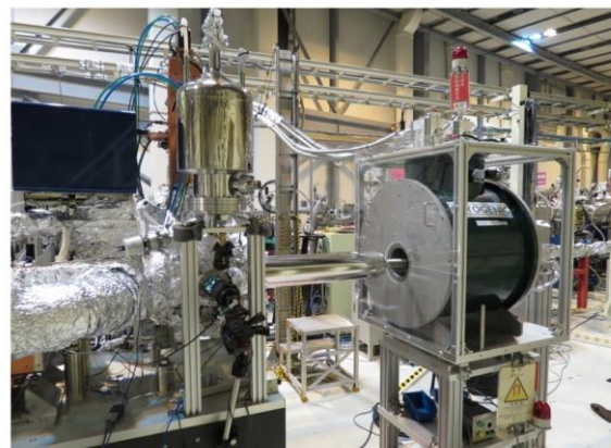
Fig. 3. New superconducting magnet for nano-XMCD at the B-branch of BL25SU.
