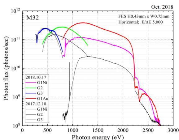
Fig. 3. Photon flux curve of BL27SU C-branch before and after the upgrade.
