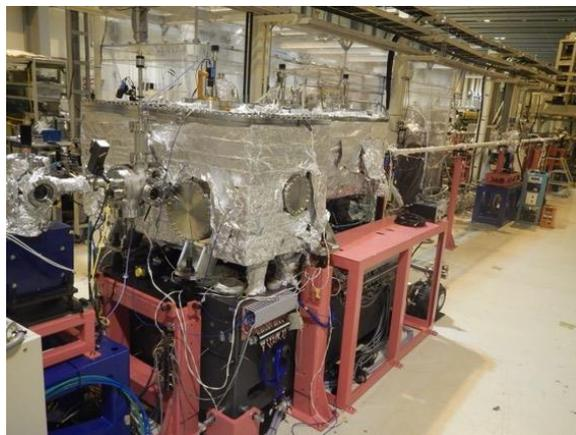
Fig. 1. Overview of new monochromator chamber installed on BL27SU.
