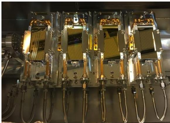
Fig. 2. Photograph of the four installed gratings with a new cooling system.
