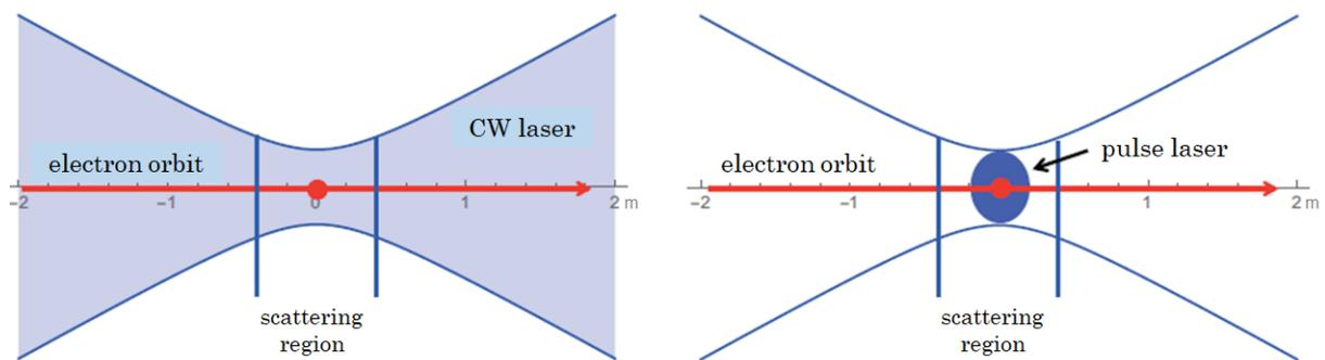
Fig. 3. Schematics of the laser Compton scattering near the collision point for (left) a CW laser and (right) a pulse laser synchronized with a beam bunch.
