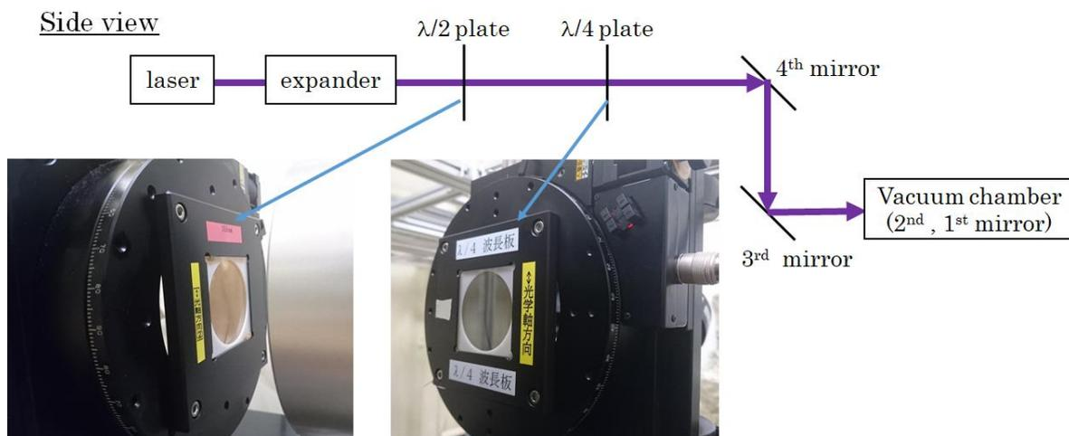
Fig. 1. Setup to inject circularly polarized laser light to the SPring-8 storage ring.
