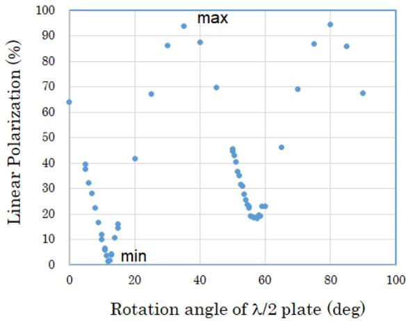
Fig. 2. Variation of the linear polarization at the laser-beam end in the SR tunnel against the rotation angle of the  $\lambda/2$  plate. Axis of the  $\lambda/4$  plate is fixed in this measurement.
