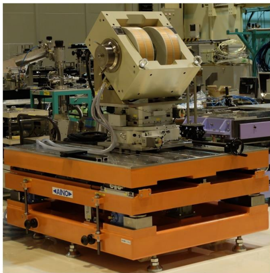
Fig. 3. New electromagnet for X-ray spectroscopy experiments under extreme conditions.
