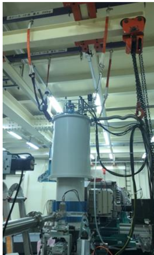
Fig. 2. 7-T cryomagnet installed on the high-resolution spectrometer.
