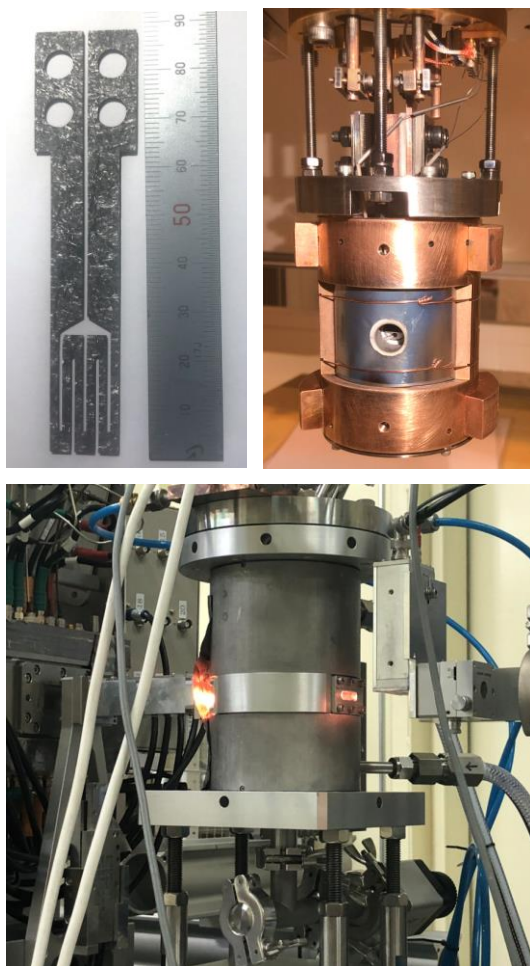
Fig. 1. High-temperature vacuum furnace. Upper left is one of the carbon composite heaters. Upper right is the sample unit before installation in the vacuum chamber. Lower panel shows the furnace in use at BL43LXU.
