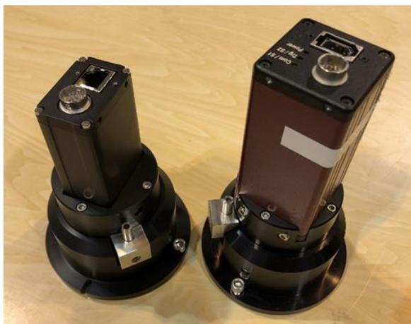
Fig. 1. Two-dimensional CCD detectors for the HAXPES analyzer. (left) high-speed detector with 70 fps, and (right) the detector with 13 fps.
