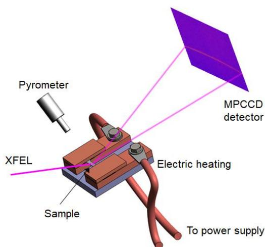
Fig. 3. Experimental setup for *in situ* XRD measurements of steel samples under ultrafast heating up to  $10^4$  °C/s.
