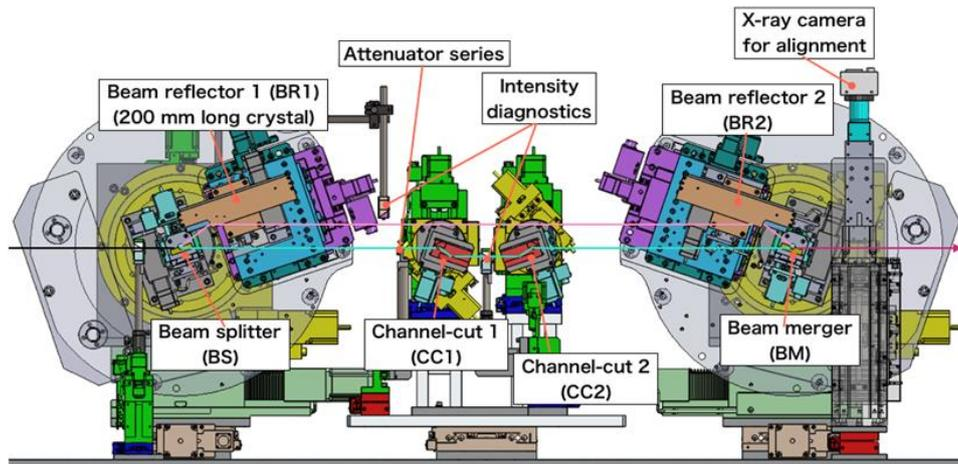
Fig. 2. Split-and-delay optical system at SACLA BL3.
