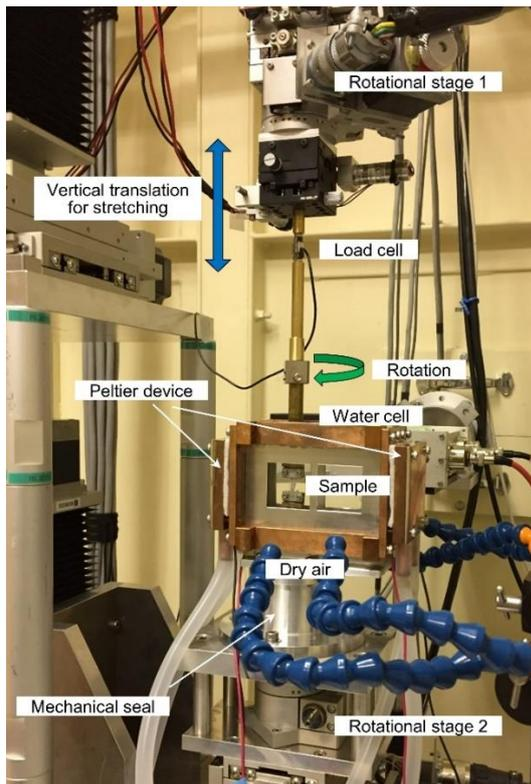
Fig. 2. Sample stage for 4D X-ray phase tomography under stretching.
