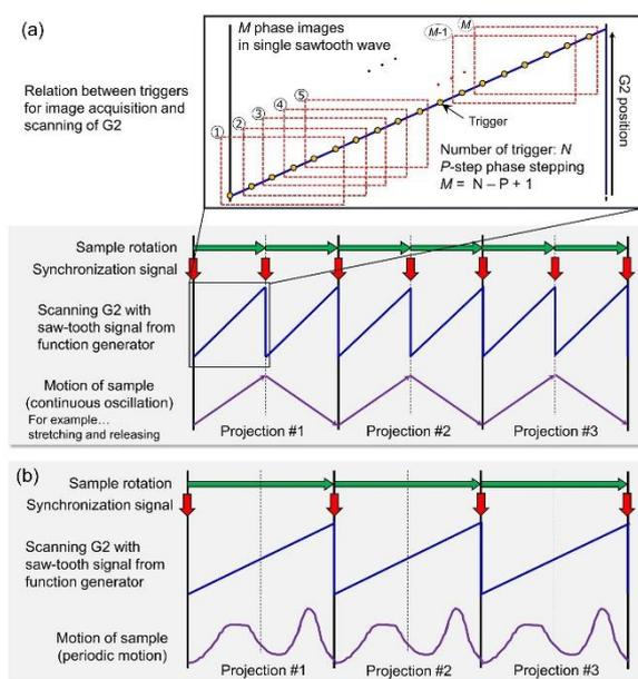
Fig. 1. (a) Schematic drawing of the scanning procedure in 4D X-ray phase tomography to observe continuously oscillating biological soft tissues. (b) Improved scanning procedure to observe more complicated periodic motion.
