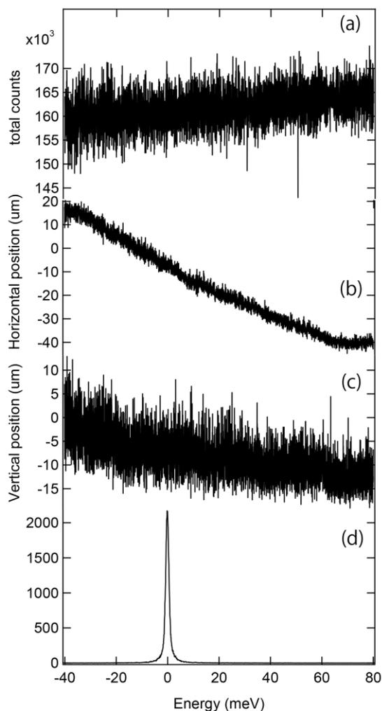
Fig. 1. X-ray position dependence with an energy scan. (a) Total flux obtained from XBPM. (b) and (c) Horizontal and vertical position shifts in the energy scan. (d) Corresponding IXS energy scan ( $-40$  meV to  $80$  meV).
