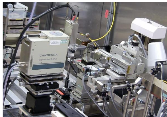
Fig. 1. Layout of the scanning microscopic XRF/XAFS measurement system.
