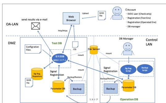
Fig. 2. Schematic of the signal registration for the parameter database.
