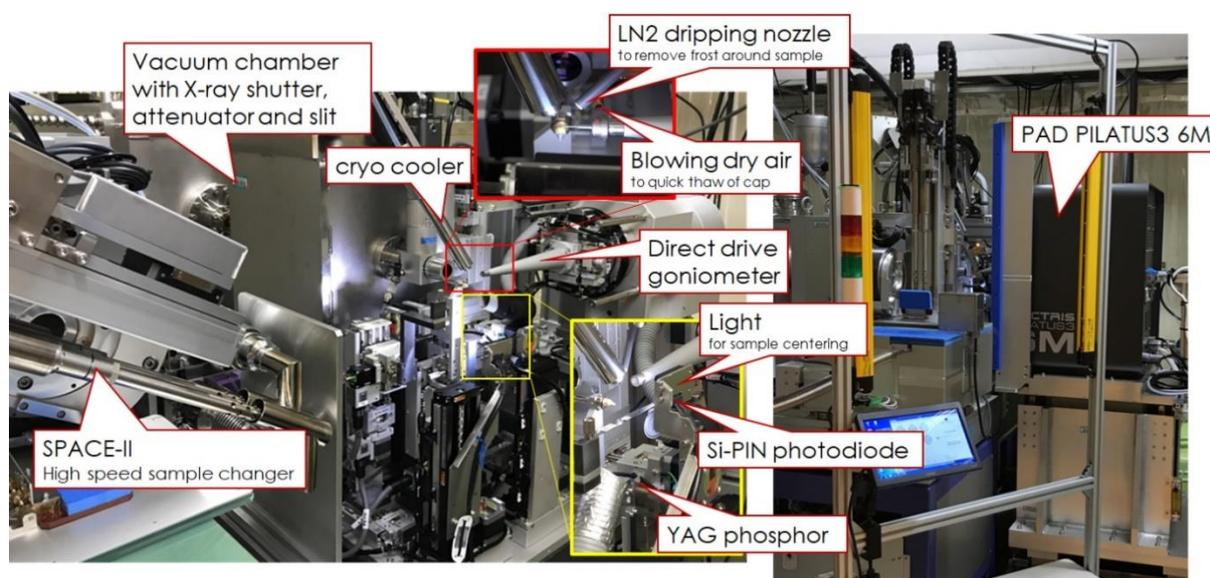
Fig. 2. Diffractometer components in the experimental hutch.
