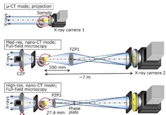
Fig. 2. Schematic diagram of multiscale-CT at BL47XU.
