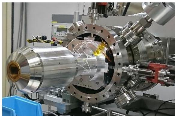
Fig. 1. Wide-angle objective lens mounted on the analyzer of BL47XU.
