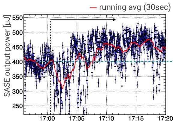
Fig. 5. SACLA accelerator parameter tuning by a Gaussian process regression.
