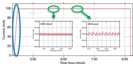
Fig. 4. Top-up beam injection from SACLA.
