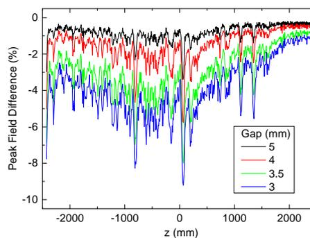
Fig. 6. Demagnetization observed for the first undulator segment of BL1.
