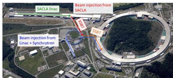
Fig. 3. Beam transport for injection (XSBT and SSBT).
