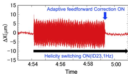
Fig. 2. Horizontal orbit fluctuation due to the helicity switching at ID23.
