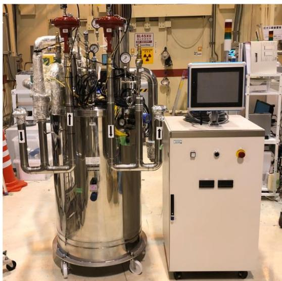
Fig. 2. New liquid-nitrogen circulators for high heat load optics.
