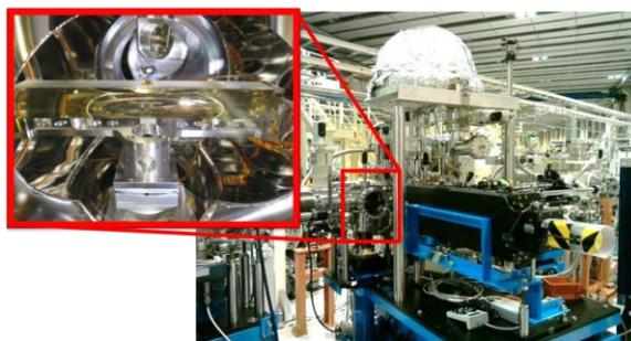
Fig. 3. Soft X-ray micro-ARPES apparatus and installed monolithic Wolter mirror at BL25SU.
