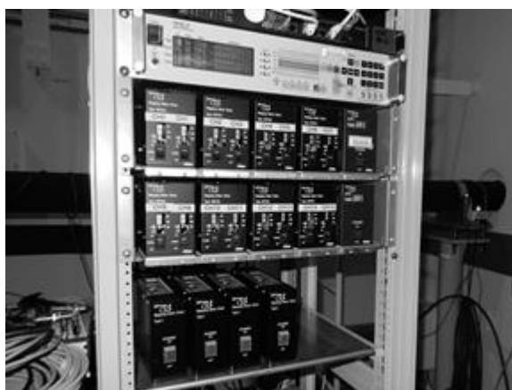
Fig. 2. Photograph of the pulse motor-driving system. Controller (PM16C-16) can be controlled through an Ethernet or USB connection.
