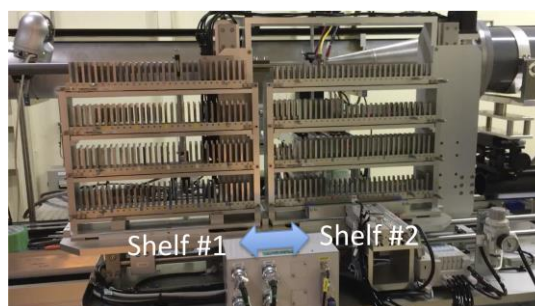
Fig. 2. Expanding unit for HummingBird for SAXS measurement in the third hutch.
