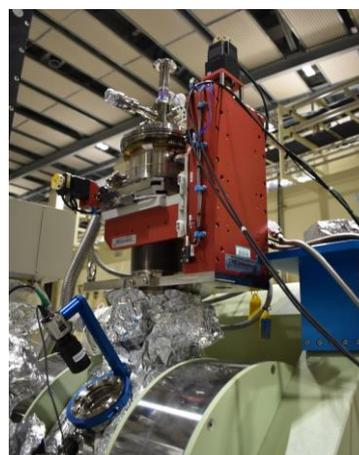
Fig. 1. Manipulator of the electromagnet-type XMCD apparatus at the B-branch of BL25SU.
