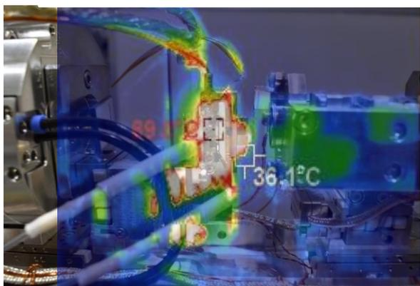
Fig. 2. High-temperature sample stage with overlaid thermal camera image for nano-XMCD at the B-branch of BL25SU.
