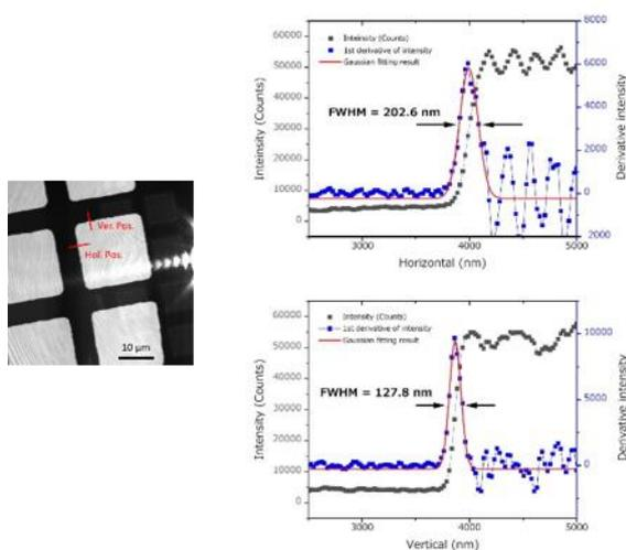
Fig. 2. Transmission image of Cu mesh obtained using the full-field TXM system (left) and horizontal and vertical intensity profiles (right).
