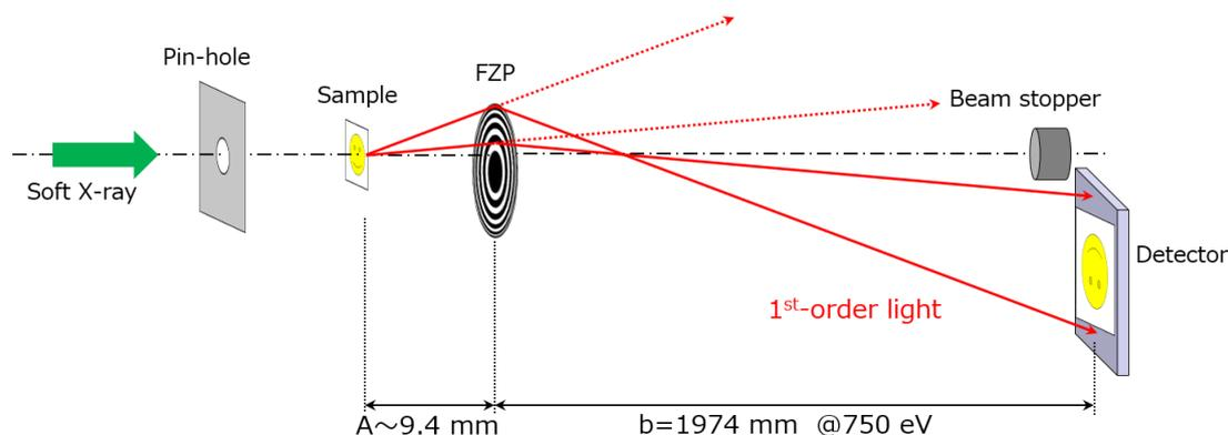
Fig. 1. Schematic view of the TXM-XAS system at BL27SU.
