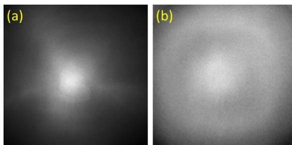
Fig. 1. Beam profile at focal point. (a) Capillary condenser and (b) BS-CZP.
