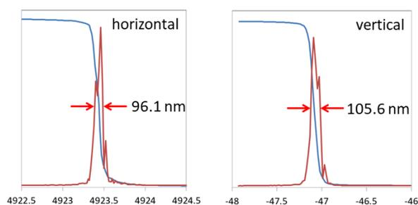
Fig. 3. Focusing beam profiles at 30 keV obtained during Ge-SSD operation.
