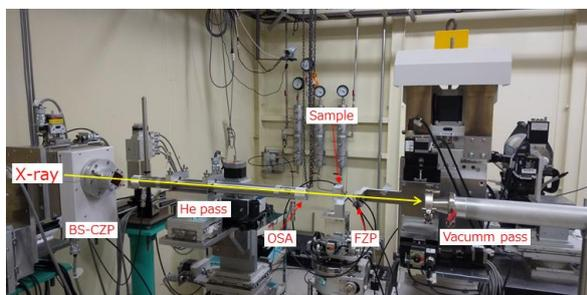
Fig. 2. Layout of full-field transmission spectroscopic imaging using BS-CZP.
