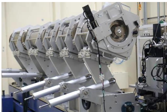
Fig. 1. WAXD setup with all the vacuum tubes and the flange flipped up.
