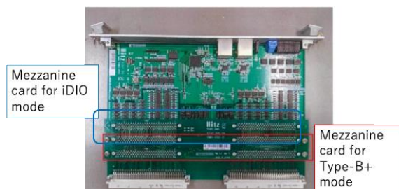
Fig. 3. I/O card with EtherCAT, red box shows Type-B+ setting and blue box shows iDIO mode.
