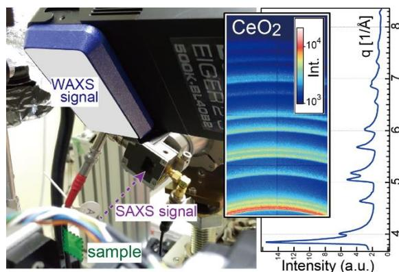
Fig. 1. WAXS detector, Eiger2 S 500K, installed at BL40XU in SAXS/WAXS simultaneous measurements. The inset figure and the figure on the right show the 2D-WAXS image obtained from the cerium (IV) oxide sample and its WAXS profile, respectively, using an incident X-ray of 15 keV. In this case, the WAXS profiles covered the Q-range of 3.7 to 8.4  $1/\text{\AA}$ .
