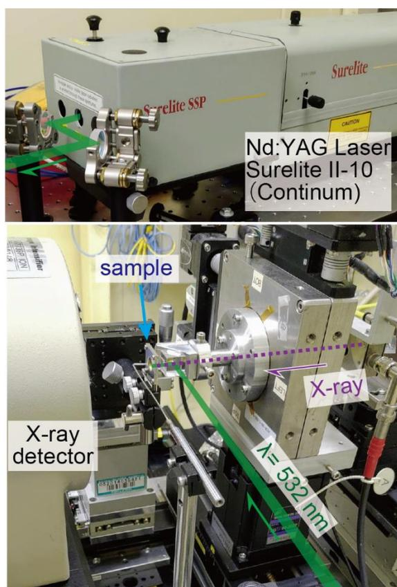
Fig. 2. Nd:YAG laser flash system in experimental hutch 1 (top) and its application to time-resolved WAXS measurement (bottom).
