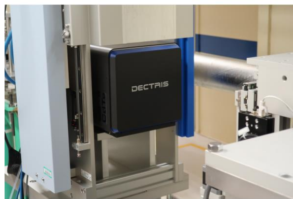
Fig. 3. EIGER2 X CdTe 4M installed in experimental hutch1.
