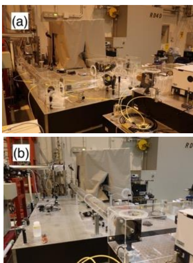
Fig. 1. (a) Old light path and (b) reconstructed light path.
