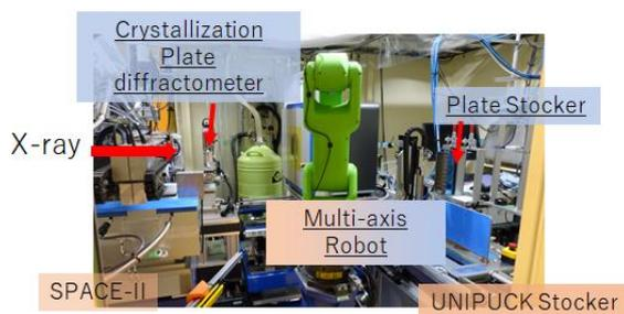
Fig. 2. Diffractometer components in Exp. Hutch.
