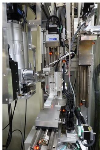
Fig. 4. Diffractometer for crystallization plate *in situ* measurement.
