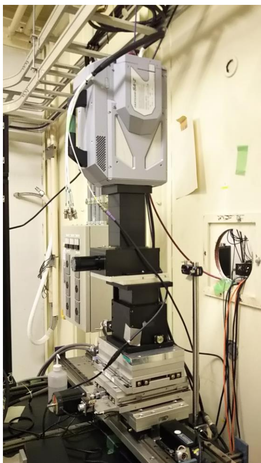
Fig. 4. High-speed X-ray image detector at experimental hutch 1.
