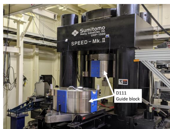
Fig. 2. D111 guide block installed on the SPEED-Mk.II.
