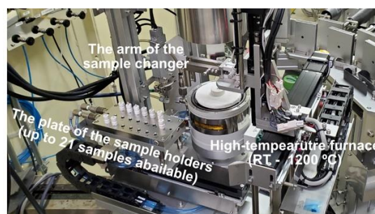
Fig. 1. Experimental setup of the horizontal diffractometer and automated sample changer with furnace in BL04B2.
