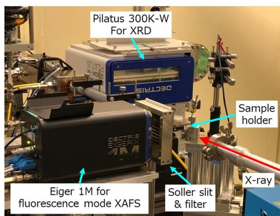
Fig. 1. Experimental setup of simultaneous time-resolved fluorescence-mode QXAFS/XRD measurement system.
