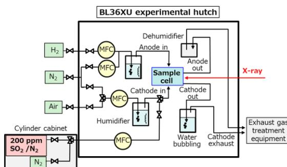
Fig. 3. Schematic layout of on-site SO<sub>2</sub> poisoning system.
