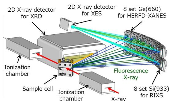
Fig. 2. Schematic layout of XES/XAFS/XRD measurement system.
