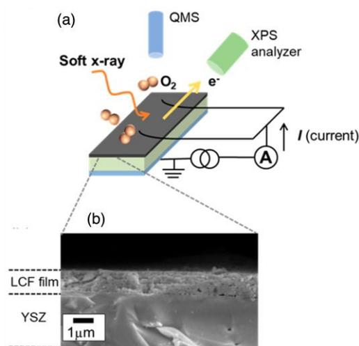
Fig. 1. (a) Schematic illustration of the *operando* XPS setup, where the applied positive current desorbs oxygen from the LCF film surface. (b) Cross-sectional scanning electron microscopy image of the prepared LCF film on yttrium-stabilized zirconia (YSZ).
