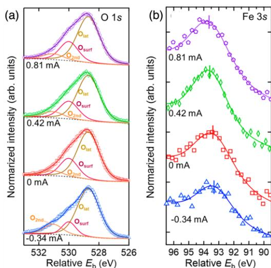
Fig. 2. *Operando* XPS spectra of (a) O 1s and (b) Fe 3s core levels in the LCF film on YSZ at 600 °C with applied currents. The photon energy was 700 eV. In (a), curve fittings of the peaks were made to decompose components of the chemical species,  $O_{lat}$ ,  $O_{surf}$ , and  $O_{2nd}$ .
