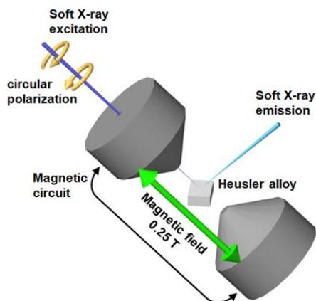
Fig. 3. Geometry of RIXS experiments under a magnetic field.
