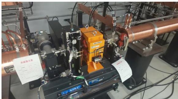
Fig. 4. Pulsed quadrupole magnet installed at a C-band main accelerator section.
