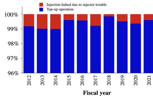
Fig. 2. SPring-8 top-up operation statistics for the past ten years. The injection from the SACLA linac started in FY2020.
