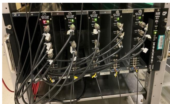
Fig. 1. Photograph of the new data processing system consisting of five APN504 modules.
