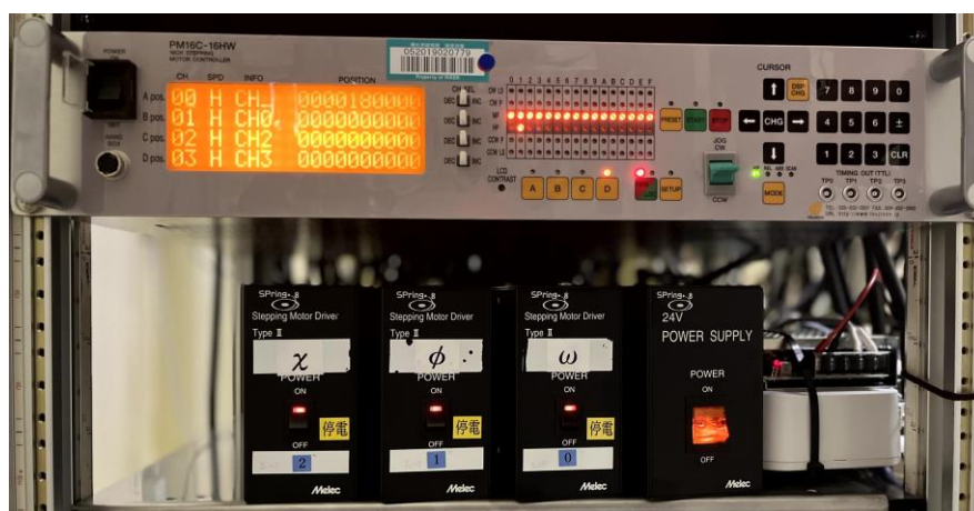
Fig. 1. New motor drivers and controller for the single-crystal X-ray diffraction measurement.
