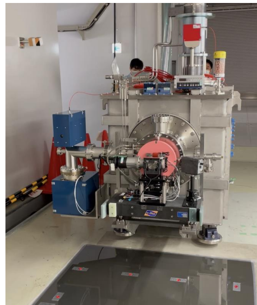
Fig. 5. New electron gun swapping system.
