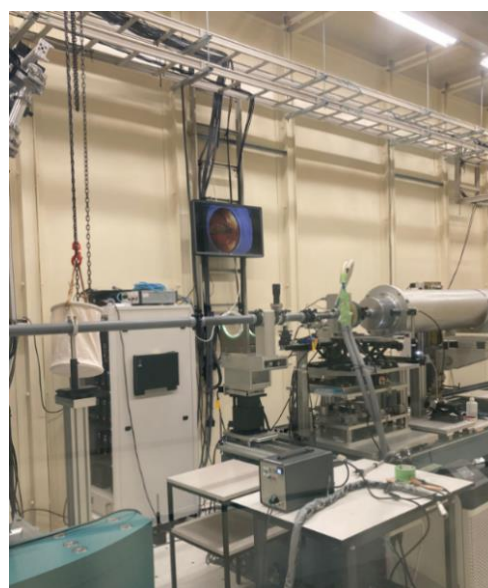
Fig. 4. Experimental setup for SAXS and WAXD simultaneous measurement.
