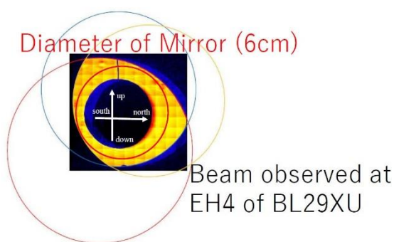
Fig. 2. Blockage of X-ray beam by the offset of multiple vacuum pipes located between EH3 and EH4 of BL29XU.
