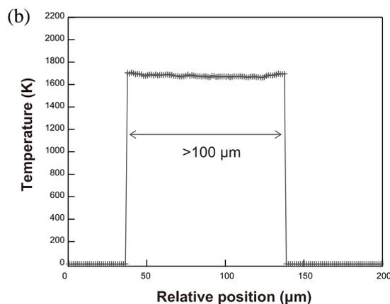
Fig. 2 (a) New optical system comprising a focal  $\pi$ -shaper (Focal- $\pi$ Shaper 9\_1964, AdlOptica) and a laser expander. (b) Temperature measurement profile of platinum foil during test heating.
