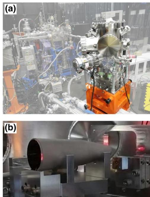
Fig. 1. (a) Photograph of the general-purpose nanofocusing apparatus equipped with (b) a focusing Wolter mirror.
